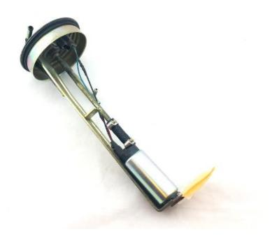
5 – reinstall the assembly into the fuel tank and attach a length of hose to the outlet of the pump assembly allowing it to drain into a fuel safe container and prime the fuel pump assembly
