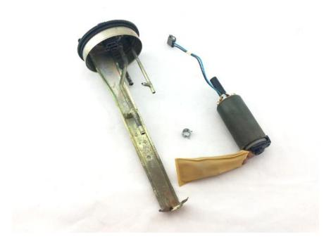
2 – prep the DW pump with components from the universal installation kit and reusable OE components.
